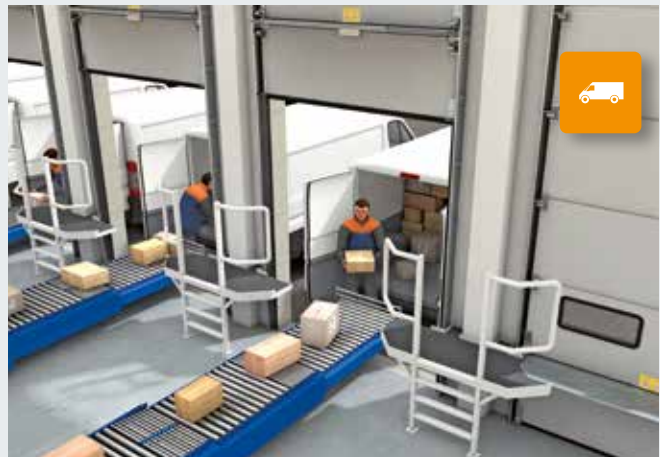
Vans are loaded at floor level. For this purpose, the door is opened completely including the bottom section.
